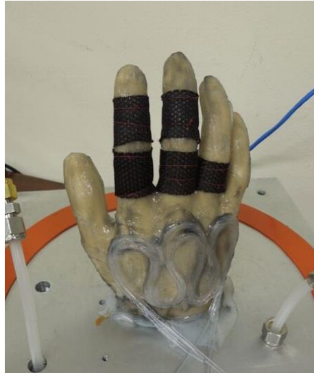
Figure 46. Partially constructed glove with exposed Bioflex and cooling matrix readied for hard vacuum testing at Paragon SDC.
