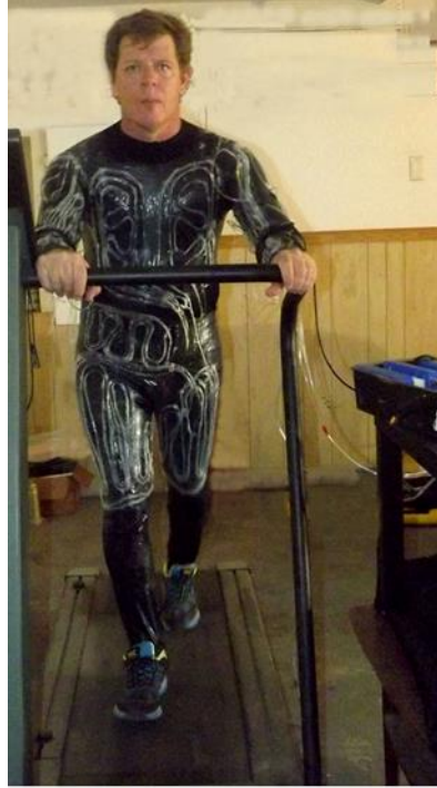
Figure 43. Cooling system testing on treadmill.
