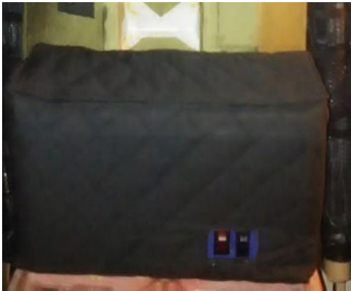
Figure 31. Padded waist pack thermal controller with activation switches.
