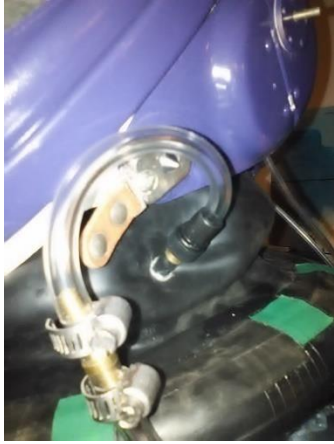
Figure57. Helmet internal pressure monitoring line detail.
