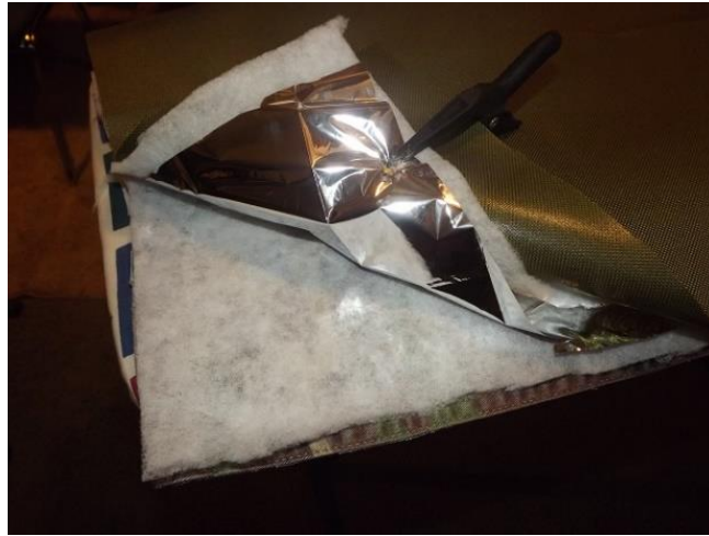
Figure 34. Alternating layers of Polyfill and Mylar thermal blanket.
