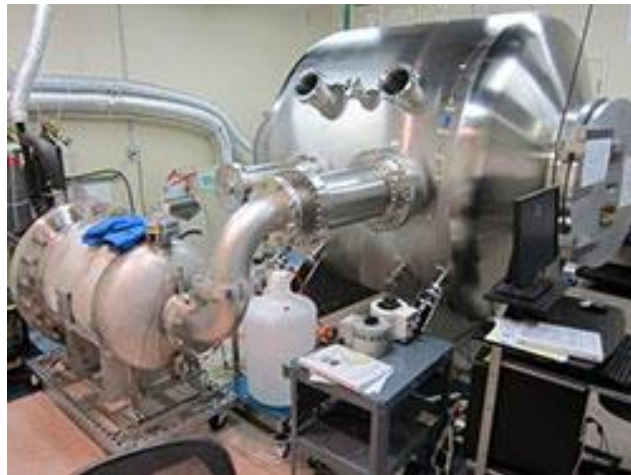
Figure 44. Paragon SDC EHF hypobaric testing chamber.
