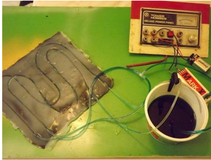
Figure 28. Flow rate testing.
