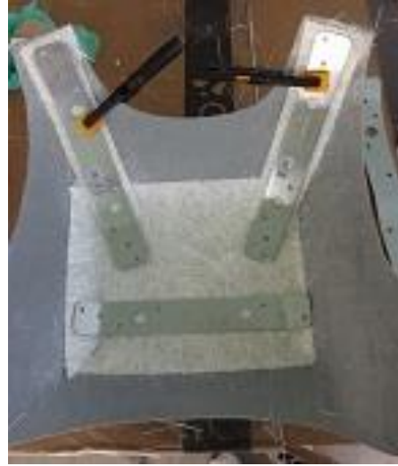
Figure 14. Hard torso fabrication and Lamination process.
