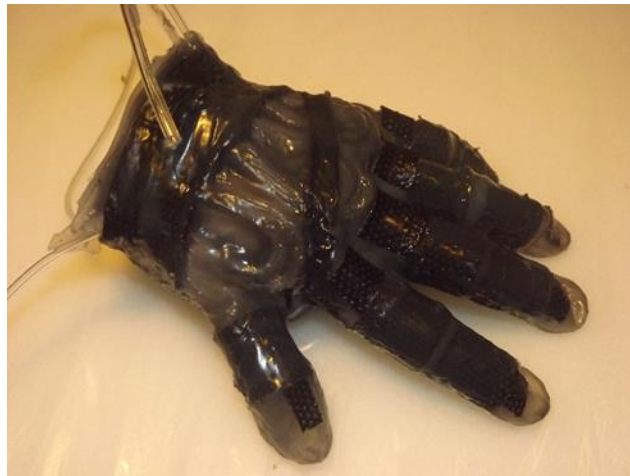
Figure 39: Completed inner liner with cooling.
