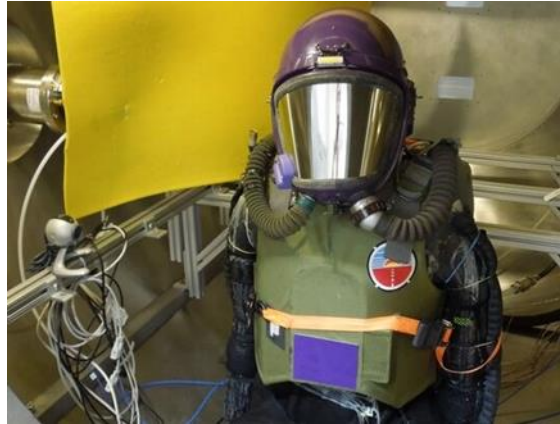
Figure 49. Transitional neck seal in EHF chamber being readied for testing.
