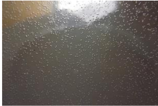
Figure 23. Chemical reaction (gas bubbles) in acrylic causing visor failure under pressure.
