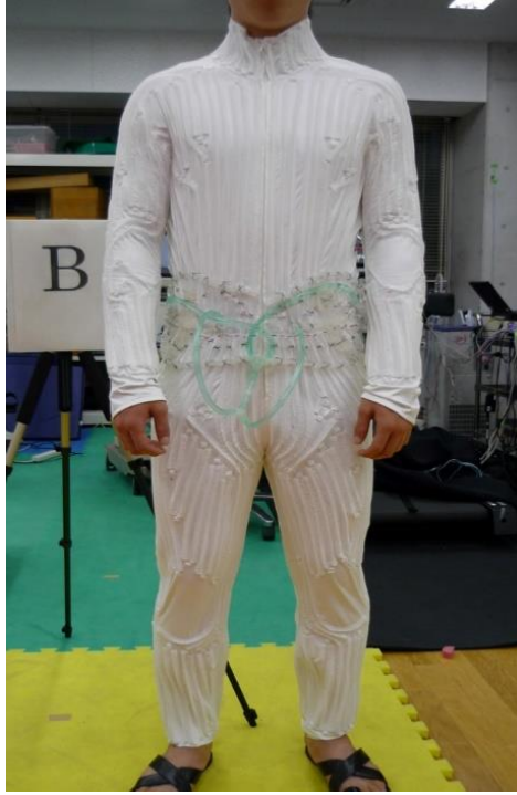
Figure 2. Liquid cooling undergarment.
