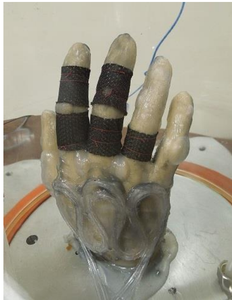
Figure 52. Partially completed glove liner in hard vacuum.
