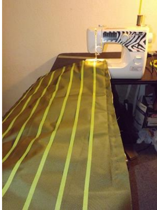
Figure 36: Stitch pattern layout with low adhesion masking tape.
